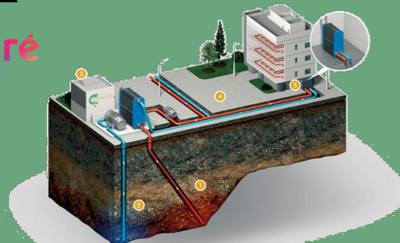
Geothermal heat production, extraction and marketing of geothermal lithium
